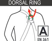
The rings marked with "A" are the only attachment points that can be used for arresting a fall! Only to these points it is allowed to connect one of the following fall arrest equipment:
